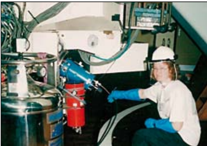
The author filling the cryostats of the IDS instrument at the Isaac Newton Telescope in 2003, complete with protective clothing.
