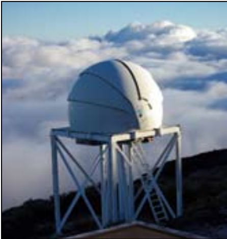
One of the DIMM telescopes which measure astronomical seeing.
