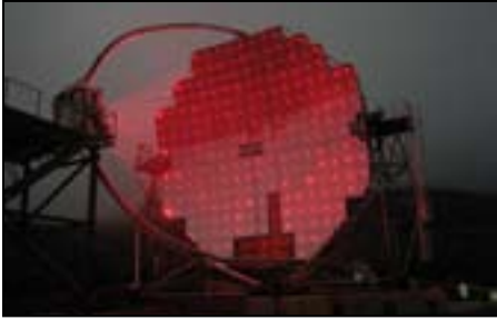
The MAGIC Telescope at night, by R. Wagner The telescope used to use lasers to align and focus the mirror segments. The laser beams could only be seen on foggy nights.
